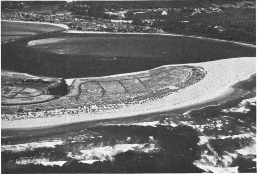
Figure 4. The southern portion of the Alsea sandspit. Note the breached foredune and developing beach berm.
